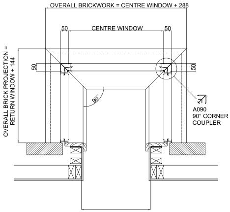
STUD OPENING = CENTRE WINDOW - 212 WITH 250 BRICK VENEER WALL STUD OPENING = CENTRE WINDOW - 162 WITH 225 BRICK VENEER WALL
