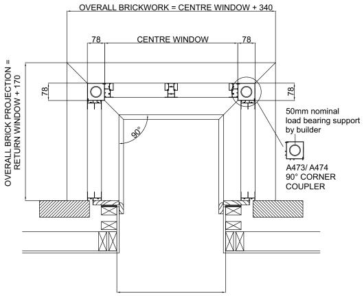
STUD OPENING = CENTRE WINDOW - 160 WITH 250 BRICK VENEER WALL STUD OPENING = CENTRE WINDOW - 110 WITH 225 BRICK VENEER WALL
