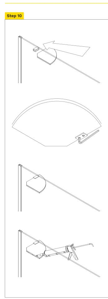
Install gusset leaving 3 mm gap off glass panel. Apply silicone between gusset and glass panel.
