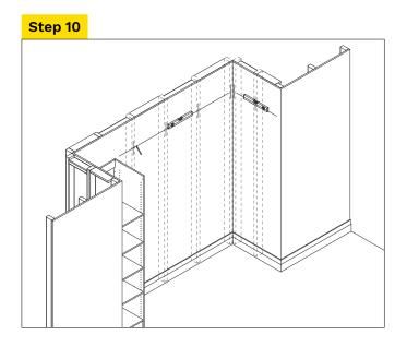
Use spirit level to mark horizontal line from top of shelf unit across full width of rear wall for back cleat and side cleat positioning.
