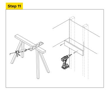
Apply liquid nails to back of side cleat in radio wave pattern and screw cleat to wall into stud.
