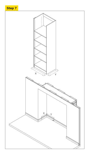
Measure the width and depth of tower and mark skirting with pencil (be sure to include the infill if infill required).
