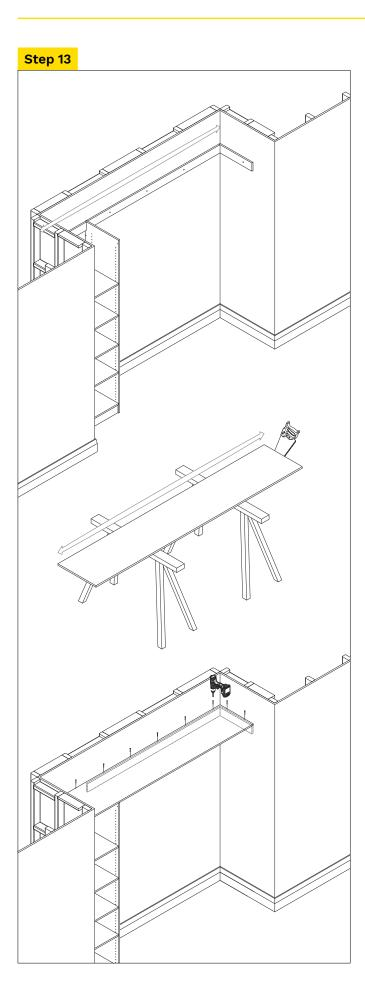
Measure top shelf width ensuring you check the walls are square using a square edge.
