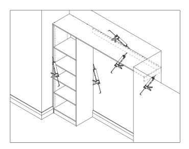
Using caulking, gap all connections between board and wall or board and board.
