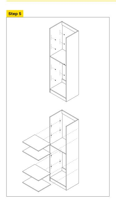
After tower has been positioned and fixed to the wall, fit shelf brackets in and place shelves at desired height.
