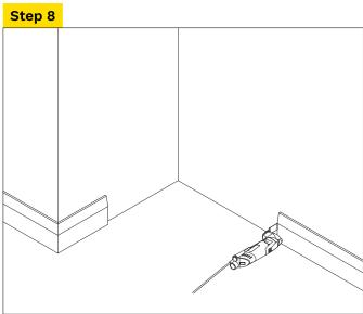
Use multi tool to cut and remove skirting where tower is to be installed.
