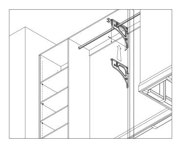
Hanging rail sharkfin support must be screwed into a stud.
