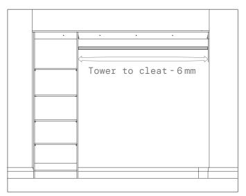
Measure distance between board (tower to side cleat) and deduct 6 mm off overall width.
