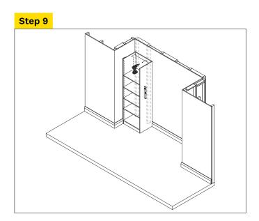
Pre-drill 2 x 3 mm holes into tower nailer. Place tower in position.
