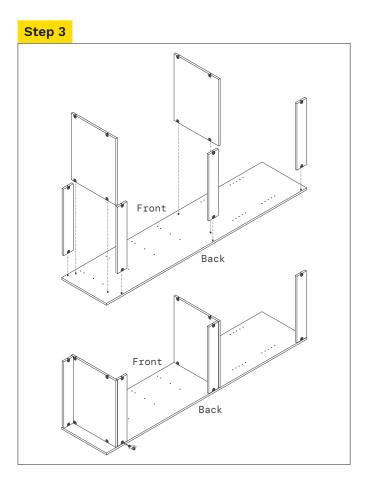
Place nailers over cam bolts and tighten. Place deck over cam bolts and tighten. Place fixed shelf over cam bolts and tighten.
