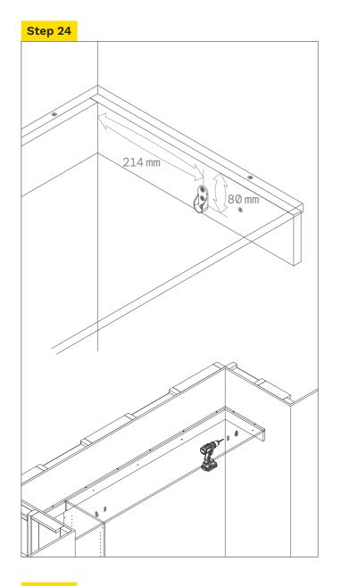
Measure 214 mm off cleat on back wall and 80 mm down from side cleat, thus measurement is to the bottom hole of hanging rod end.
