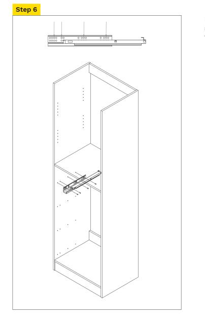
Fix runners L (B) and R (H) to tower sides, screwing euro screw into third hole in top row (Exploded image).
