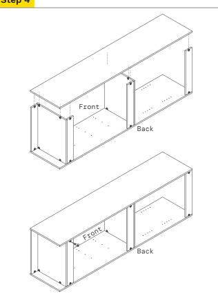
Place side on top over cam bolts and tighten cams.
