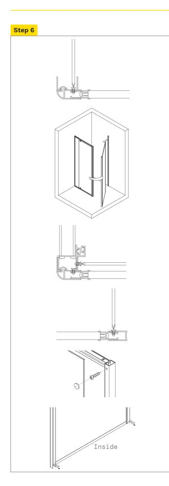
Attach side frame to return panel before completing assembly.
