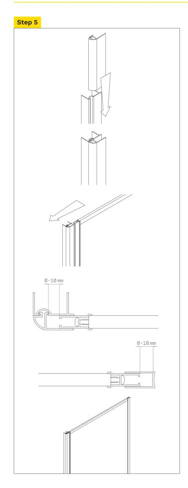
Engage 90-degree adapter to the F channel.
