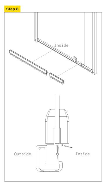
Fit seals to bottom of door ensuring angle flaps are facing inside.
