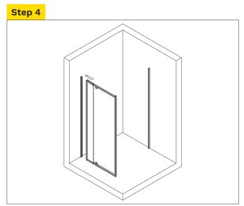
Install one side of showerscreen door panel into wall channel.
